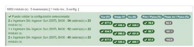
Figure 9. Configuration and number of the inverters used.
