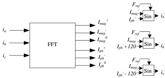
Fig. 4 FFT based algorithm for unbalance extraction
