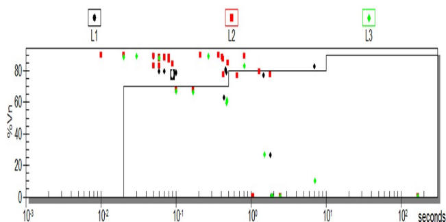
Figure 12. ITIC curve generated by the Circutor meter.
