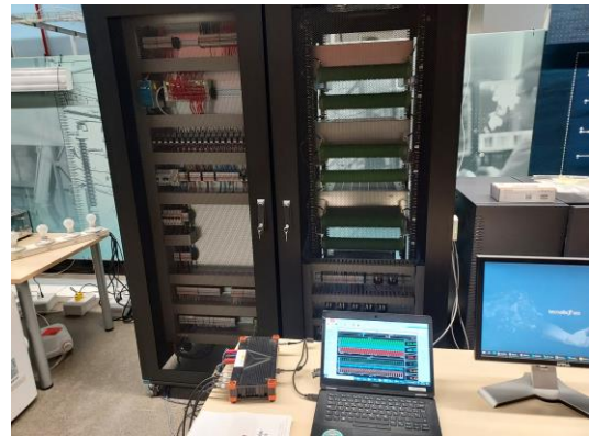
Figure 7: The control PC, the DAqS and the control devices in the cabinet
