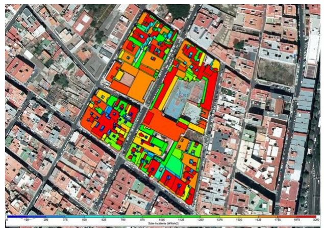
Fig.8. Aerial photo of the study area in El Toscal, with incident irradiation normalized by roof surface ( \text{kWh/m}^2 \cdot \text{year} ) with the Meteonorm corrected climate file.
