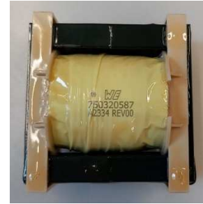
Fig.4. The transformer under test (WE 750320587 A2334 REV00)
