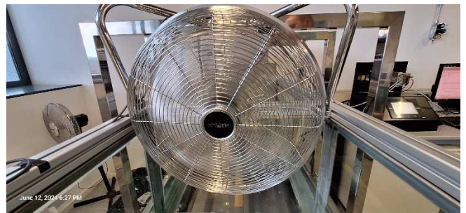
Fig. 2. In parallel to the wave generator, a fan capable of generating wind was added.
