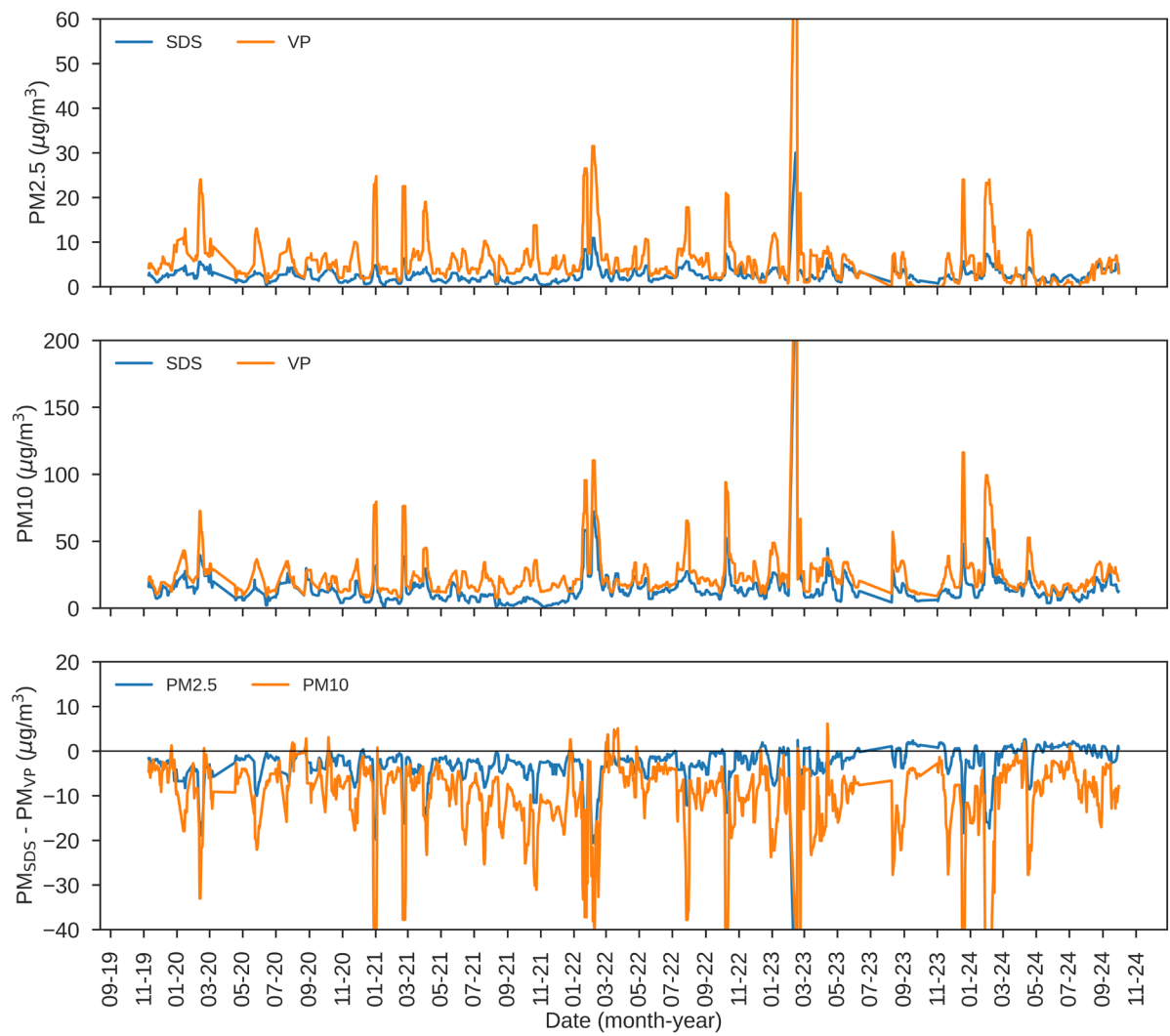
Fig. 1. PM 2.5 (top) and PM 10 (mid) concentrations from the SDS and VP datasets. The difference between these measurements is shown in the bottom panel.
