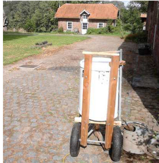
Fig. 5: A dump resistor for weed killing
