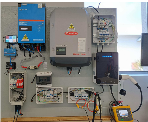
Fig. 3. The board employed in the experimental tests for the Hybrid system.
