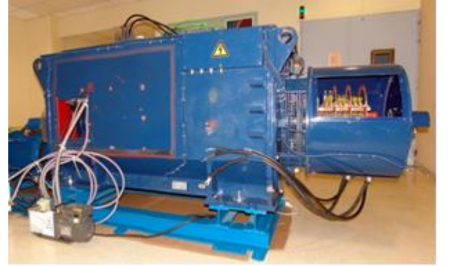
Fig 6. First 2MW class superconducting generator for medium power wind turbines [6].
