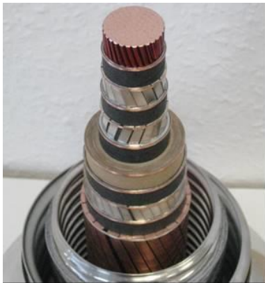
Fig. 2. Medium voltage superconducting power cable (Endesa Supercable Project, 3.2 kA, 138 MVA) [4].
