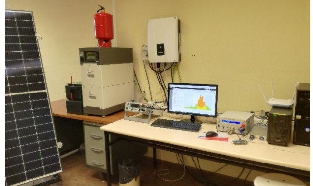
Fig. 8. Experimental LiFePO 4 Battery Cycling System. Simulation of a stand-alone/on-grid Photovoltaic applications.
