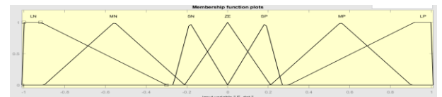
Fig. 9. Optimized membership functions corresponding to the derivative of the error signal ( \dot{e} )
