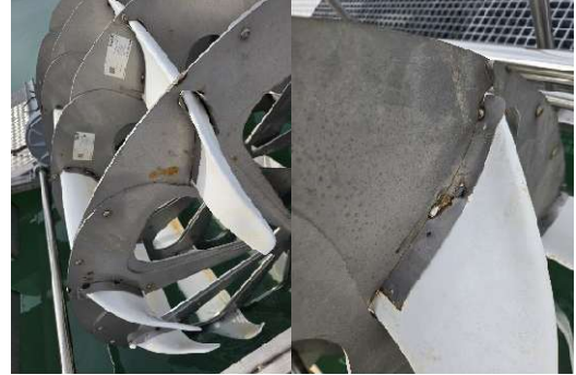
Fig. 7. Turbine blade surfaces after sustained operation, showing absence of biofouling due to continuous rotor motion.
