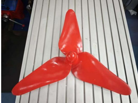
Fig. 1. Rotor designed for low-velocity conditions
