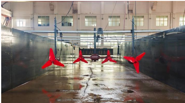
Fig. 7. Four-turbine arrays experiment layout
