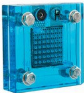
Fig. 2. Commercial PEM electrolyzer used in the educational kit.
