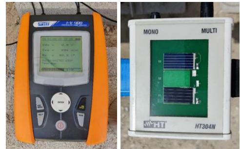
Fig. 2. Measurement equipment used in Analysis 1: (a) I-V tracer HT I-V 400; (b) irradiance meter HT304N.
