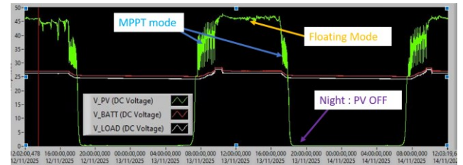
Fig. 7 Two-day visualisation of variables (here, system 2 voltages)
