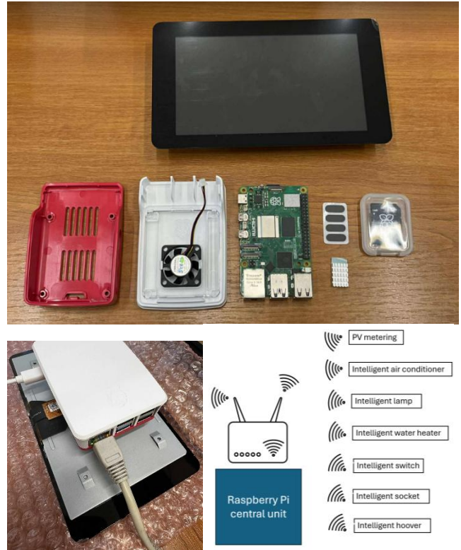
Fig. 2. The Raspberry Pi central unit
