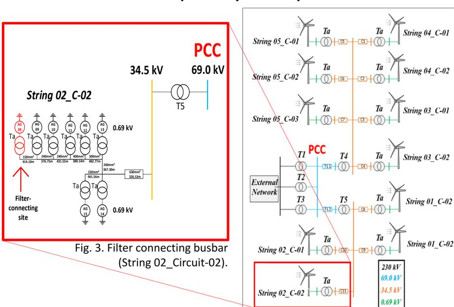
Fig. 3. Filter connecting busbar (String 02\_Circuit-02).
