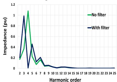
Fig. 5. Impedance-frequency response before and after connecting the 4th order tuned filter.
