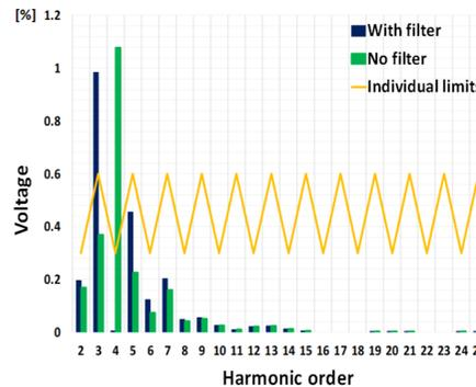
Fig. 4. Voltage harmonic spectrum before and after connecting the 4th order tuned filter.
