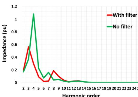
Figure 7. Impedance-frequency response before and after connecting the 7th order tuned filter.
