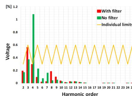
Figure 6. Voltage harmonic spectrum before and after connecting the 7th order tuned filter.
