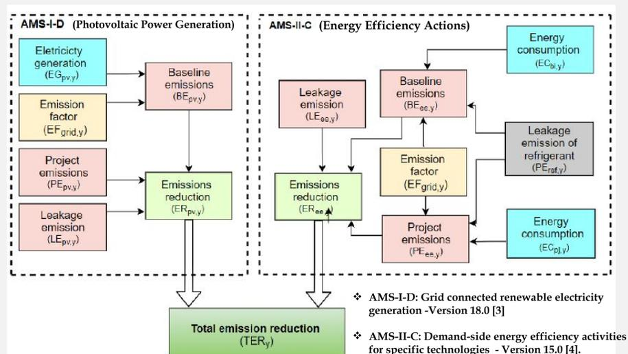
Fig. 2. Flowchart of the methodology used to quantify the reduction of CO<sub>2</sub>e emissions from the project
