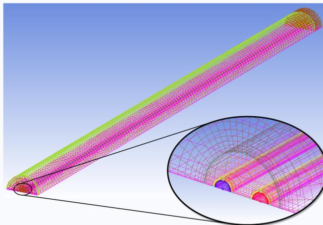
The model simulates the TRT test, where the inlet fluid and undisturbed ground temperatures are the boundary conditions. The outlet fluid temperature simulated is compared with that measured through the Root Mean Square Error (*RMSE*).
