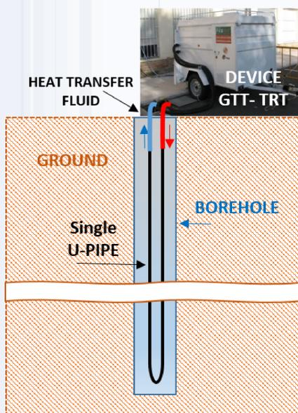
In-situ tests GTT and TRT records the undisturbed ground temperature over depth and the inlet and outlet fluid temperature along time, respectively.
