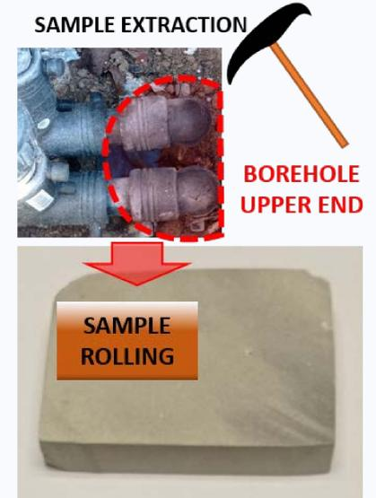
A thermal conductivity analysis over the filling material samples allowed to determine their thermal conductivity and specific heat. Density was obtained after weighing the samples, and so, the volumetric heat capacity.
