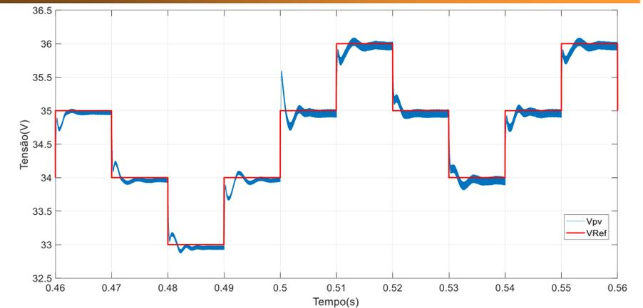
Fig 4 - Reference voltage (VRef), being disturbed by P&O, and the voltage at the terminals of the photovoltaic panel (Vpv) - Action of the IMC Controller.
