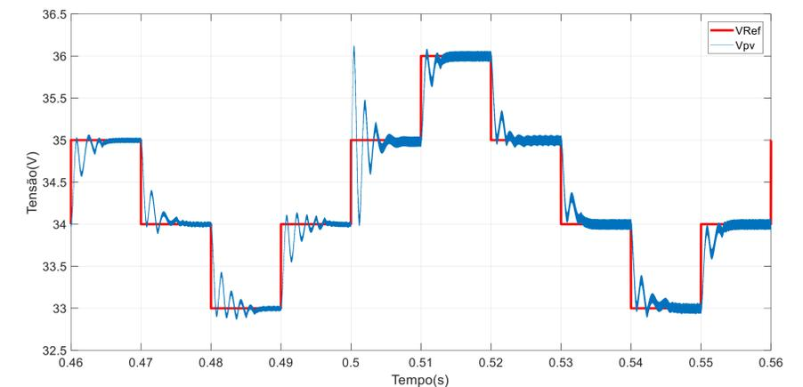
Fig 3 - Reference voltage (VRef), being disturbed by P&O, and the voltage at the terminals of the photovoltaic panel (Vpv) - Action of the PI compensator.
