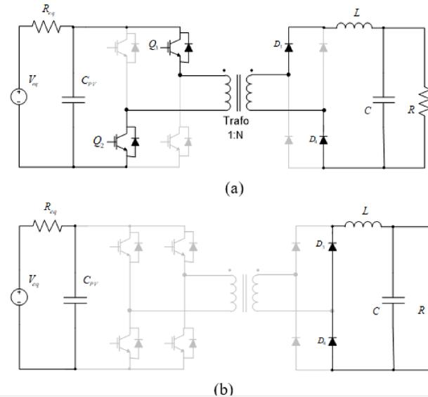
Fig. 2. DC-DC converter steps at both switching intervals..
