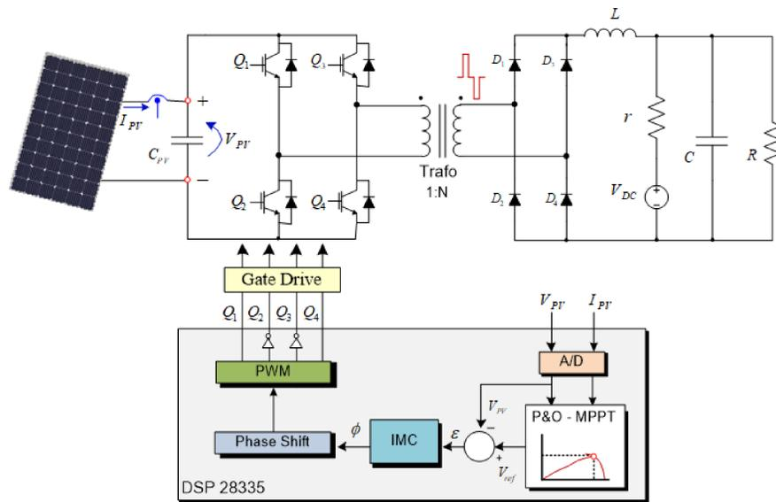
Fig.1. System structure involving MPPT, IMC controller and Full-Bridge DC-DC Converter
