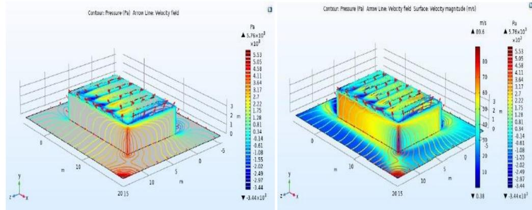
Fig.4. Wind pressure acting on the building at 225°
